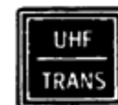
DETAIL G RSO'S CONTROL TRANSFER SWITCH
