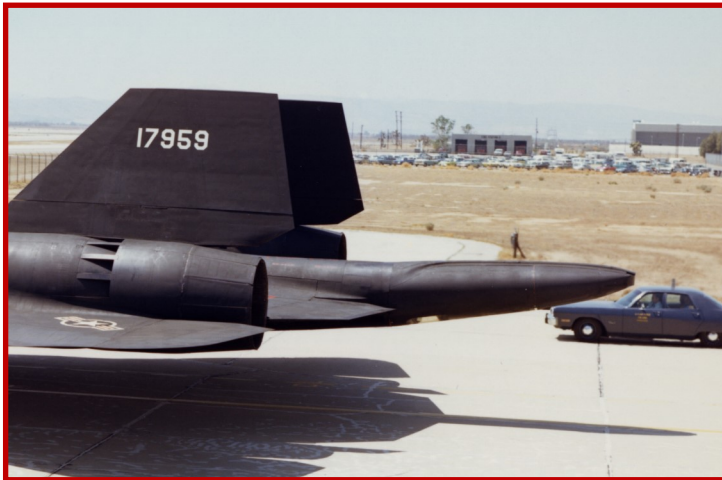
Close-up shot of the extended tail assembly on 959 as it taxi's by the camera on its way out for another test mission. The panoramic window for the Optical Bar Camera is visible on the underside of the movable tail.
