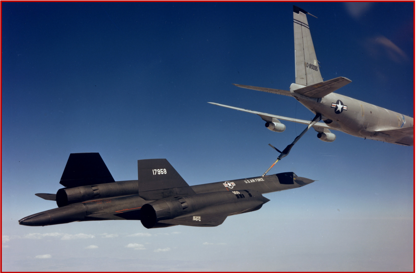
The modified tail assembly shows up well in this view as SR-71A 61-7959 'Big Tail' takes on fuel from a KC-135Q tanker aircraft. The extended tail required the fuel dump port to be routed across the top of the new tail assembly.
