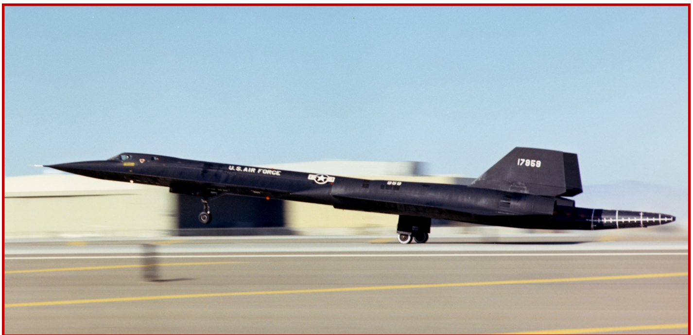
'Big Tail' departs Palmdale on another test mission. Early test flights were conducted with white calibration stripes painted on the tail to aid in tracking.
