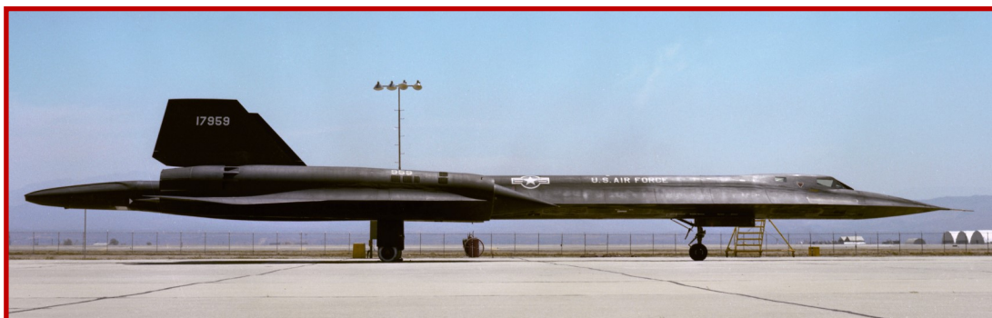
Direct side view of '959 with the new tail assembly installed sitting on the ramp at Palmdale.
