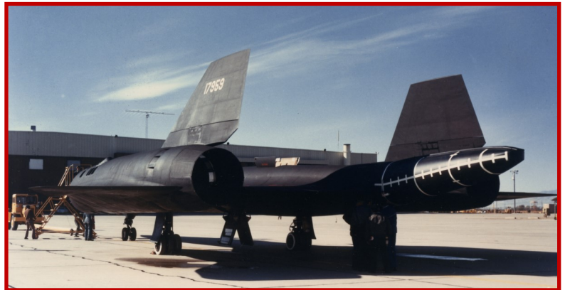
For early taxi and flight tests, calibration stripes were painted on the tail to aid in tracking.
