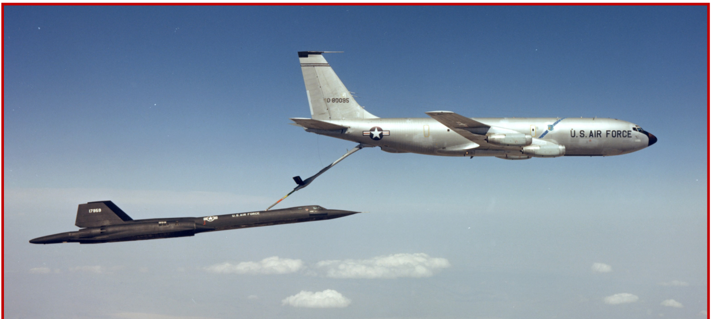
The 'Big Tail' SR-71A (61-7959) takes on fuel from a KC-135Q tanker out of Beale AFB. All 'Big Tail' test flights were flown out of Palmdale. The extended tail was used to house an Optical Bar camera as well as a variety of aft facing ECM systems.
