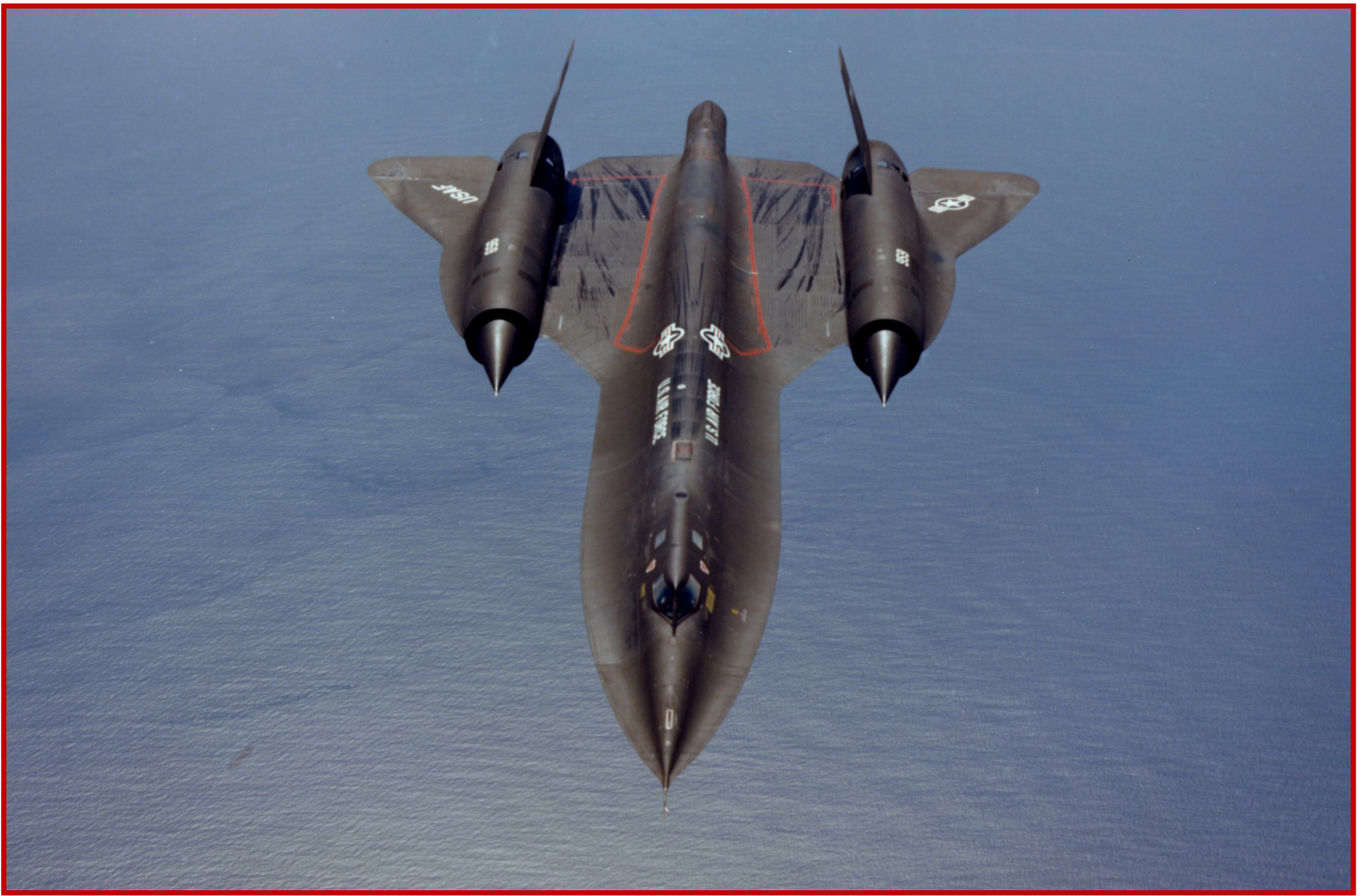
A view from the tanker looking down on 'Big Tail' off of the California coastline. In addition to the extended tail, chine bays were enlarged to house Optical Bar Cameras as an additional optical camera capability.
