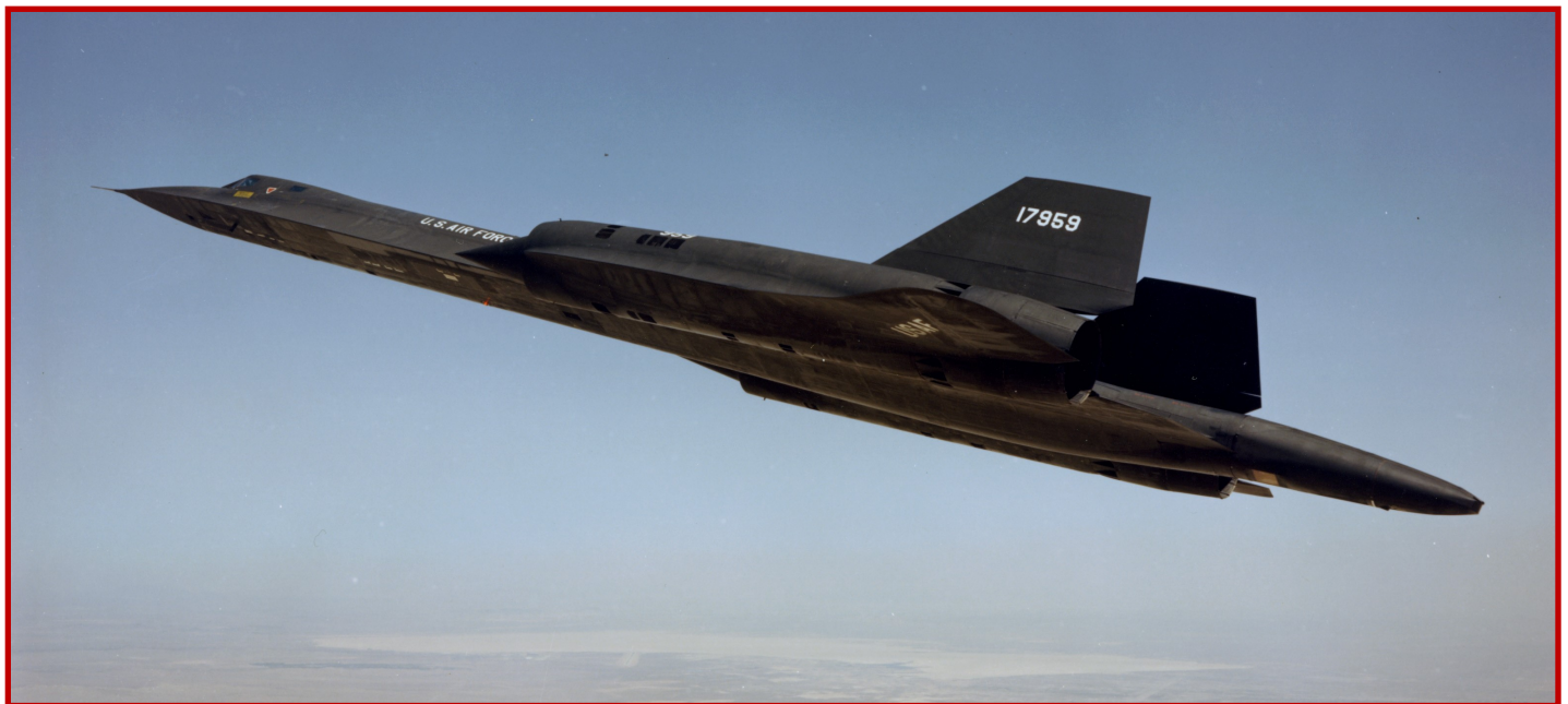
Barely visible in this view of 'Big Tail' is the optical bar camera window and aft-facing ECM antennae in the modified tail assembly as the aircraft flies in the vicinity of Edwards AFB, CA.
