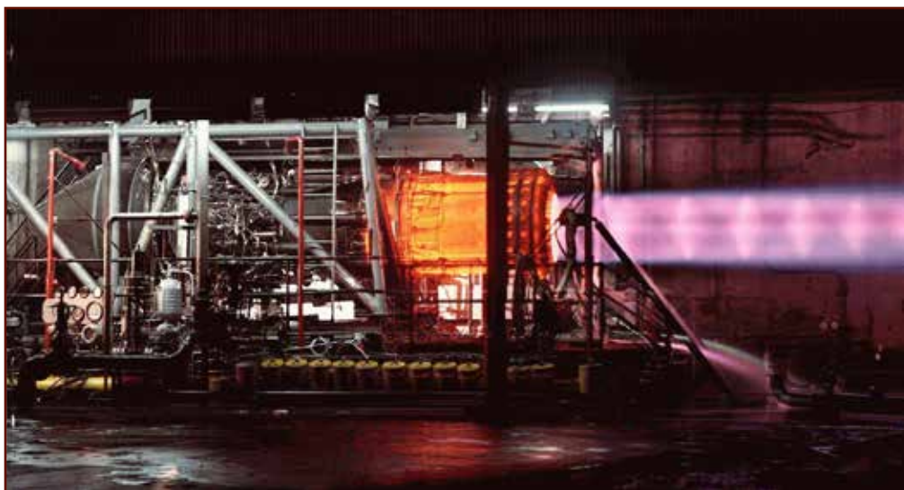
The J58 jet engine during a static test. A modified version of an engine designed for another program four years earlier, the jet generated as much power as the turbines of the ocean liner the Queen Mary.
