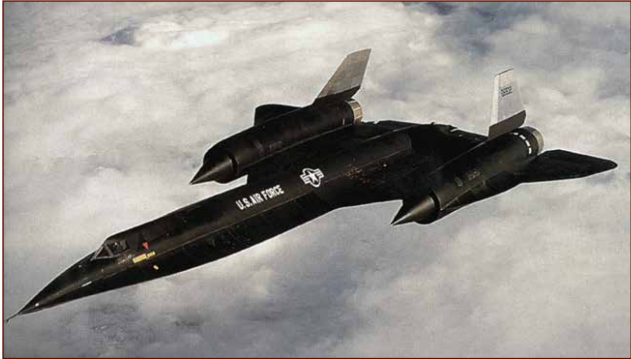
In this photo, one of the first of the A-12 released by CIA, the adjustable inlet cones in front of the engines are clearly visible. Called “spikes,” the devices regulated the incoming air flow to maximize thrust and prevent interruptions in fuel combustion at high speeds.
