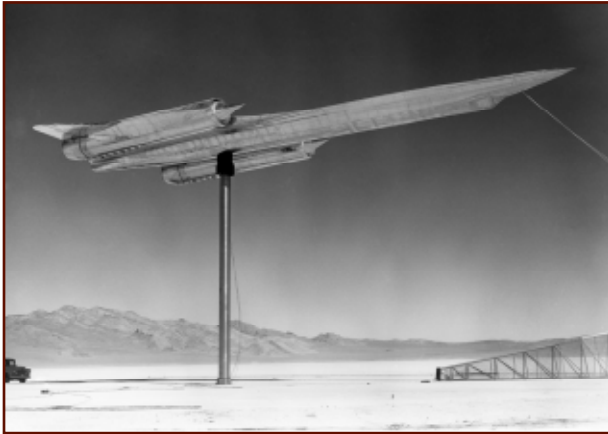
To test its radar cross section, a full-size model of the A-12 was placed in various positions on a pylon as radar readings were taken.
